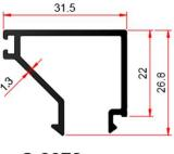
S 8372 GLAZING BEAD FOR 8MM GLASS 0.333 KG/M
